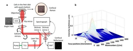
**Figure 1.** (a) Schematic of high-speed confocal Raman microscopy system; and (b) axial resolution test by moving a  $1-\mu m$  diameter polystyrene bead through the focal plane.
